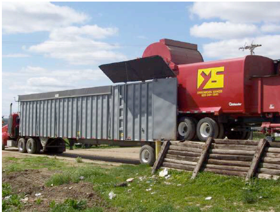
Figure 2. Keith's 53' walking floor truck trailer with truck. The trailer is shown during loading by a wood chipper. www.wilkens-ind.com/inventory/amtphoto.ashx?id=2131691&img=1
